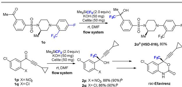
**Scheme 2.** Application of flow trifluoromethylation for the preparation of pharmaceuticals, HSD-016 and Efavirenz. <sup>a</sup>A mixture of diastereomers was obtained (the ratio was not determined). <sup>b</sup><sup>19</sup>F-NMR yield.
