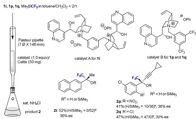
**Scheme 3.** Enantioselective trifluoromethylation of **1i**, **1p** and **1q** by a flow system. <sup>a</sup>Mixtures (R=H and SiMe<sub>3</sub>) were obtained, and ratios were determined by <sup>19</sup>F-NMR.
