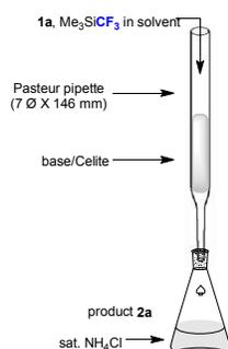
**Figure 3.** System diagram of flow reactor for trifluoromethylation.
