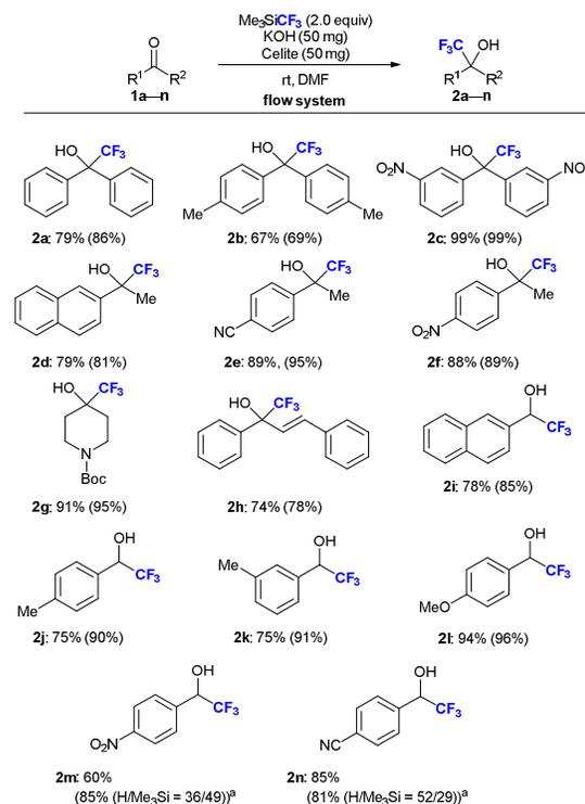
**Scheme 1.** Trifluoromethylation of carbonyl compounds **1** by the flow reaction. The values indicate isolated yield after desilylation and the values in parentheses are  $^{19}\text{F}$ -NMR yields. <sup>a</sup>LiOAc was used instead of KOH.
