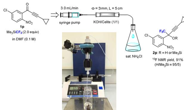
**Figure 4.** System diagram of microflow reactor for trifluoromethylation of **1p** to **2p**.
