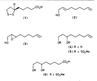
resulted in formation of the (3S)-acid (6) in 78% yield. Disulphide displacement of the methanesulphonate groups of the potassium salt of the (3S)-acid (6) proceeded with inversion of configuration<sup>11</sup> at C-3 to give (R)-(+)- $\alpha$ -lipoic acid, (+)-(1), m.p. 44–46 °C,  $[\alpha]_{D}^{25}$  +107° (c 0.82, C<sub>6</sub>H<sub>6</sub>) in 52% yield {lit. values:<sup>3</sup> m.p. 43–45 °C,  $[\alpha]_{D}^{23}$  +102° (c 0.91, C<sub>6</sub>H<sub>6</sub>)}.
