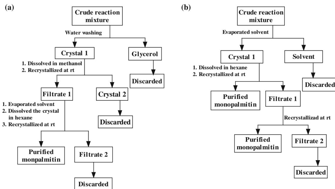
**Fig. 2** Purification of monopalmitin synthesized by the two enzymatic methods corresponding to the two reactions outlined in Fig. 1
