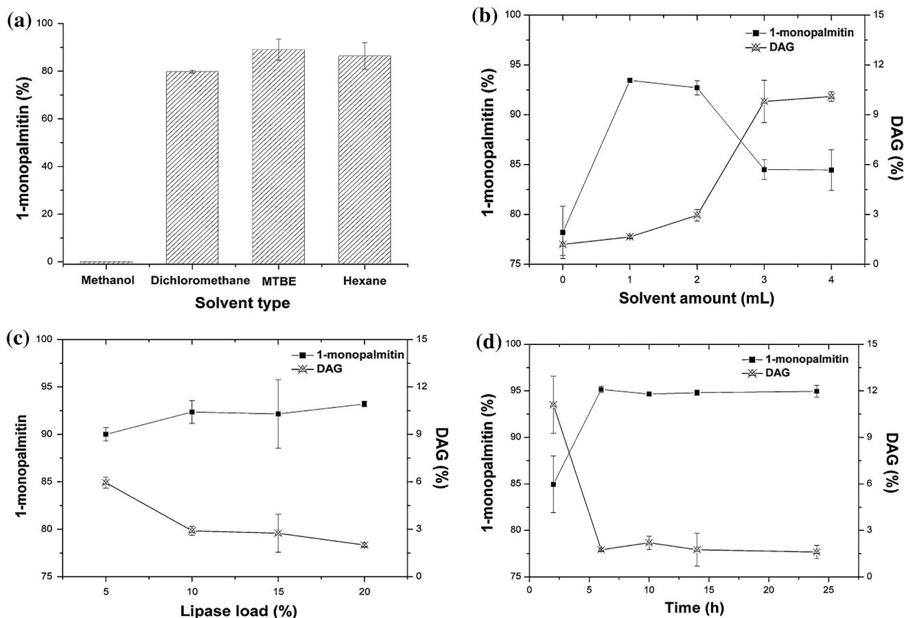
**Fig. 3** Optimization of enzymatic synthesis of monopalmitin, illustrating the effect **a** solvent type, **b** solvent amount, **c** enzyme load, and **d** reaction time
