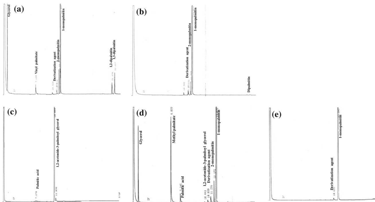
**Fig. 4** GC chromatograms of synthesis products on large scale. **a** Enzymatic synthesis of monopalmitin before purification, **b** enzymatic synthesis of monopalmitin after purification, **c** enzymatic synthesis of 1,2-acetonide-3-palmitoyl glycerol before purification,
