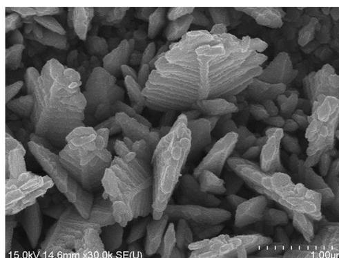
Fig. 8 SEM image of the  $\text{Co}_3\text{Ni}$  array after 6 cycles.
