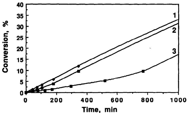
Figure 5. The effect of the amount of the salt hydrate present ( $\text{Na}_2\text{SO}_4 \cdot 10 \text{H}_2\text{O} / \text{Na}_2\text{SO}_4$ ) for the esterification reaction of fig. 1, 1g (1), 10 mg (2) and 0 mg (3).
