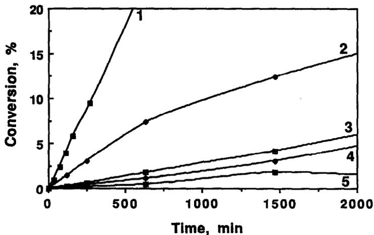
Figure 4. The effect of presence of salt hydrates ( $\text{Na}_2\text{SO}_4 \cdot 10 \text{H}_2\text{O} / \text{Na}_2\text{SO}_4$ ) when changing the organic solvent in the esterification reaction of fig. 1. Hexane with salt hydrate (1), toluene with salt hydrate (2) and without (4), diisopropyl ether with salt hydrate (3) and without (5).
