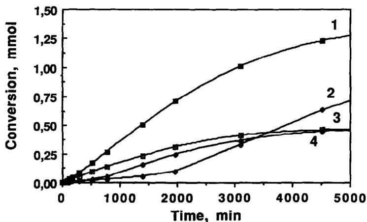
Figure 3. The effect of presence of salt hydrates ( $\text{Na}_2\text{SO}_4 \cdot 10 \text{H}_2\text{O} / \text{Na}_2\text{SO}_4$ ) when increasing the concentration of reactants in the esterification reaction of fig. 1. Three times concentration of fig. 1 with salt hydrate (1) and without (2). Same concentration as in fig. 1 with salt hydrate (3) and without (4).
