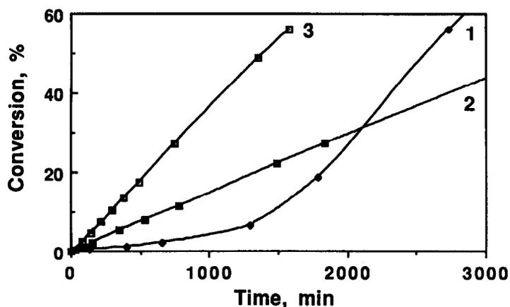
Figure 1. Esterification of butanoic acid (0.50 mmol) with butanol (1.0 mmol) catalysed by lipase (5.0 mg) from *Candida rugosa* in hexane (8 mL) (Model reaction). Nothing added (1), 6  $\mu$ L water added (2) and in the presence of 1 g of  $\text{Na}_2\text{SO}_4 \cdot 10 \text{H}_2\text{O} / \text{Na}_2\text{SO}_4$  (3).
