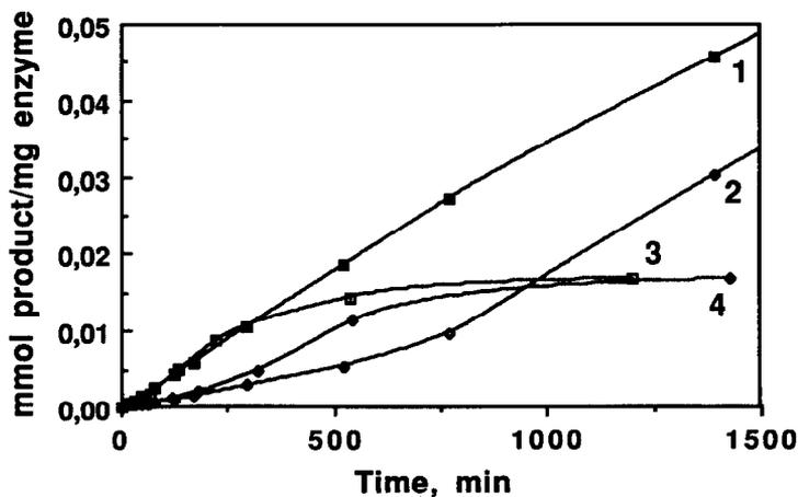
Figure 2. The effect of presence of salt hydrates ( $\text{Na}_2\text{SO}_4 \cdot 10 \text{H}_2\text{O} / \text{Na}_2\text{SO}_4$ ) when increasing the quantity of enzyme for the esterification reaction of fig. 1. 5 mg enzyme with salt hydrate (1) and without (2), 30 mg enzyme with salt hydrate (3) and without (4).
