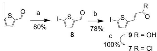
**Scheme 2.** Reagents and conditions: (a) NaO<sub>4</sub>, I<sub>2</sub>, H<sub>2</sub>O, CCl<sub>4</sub>, HOAc, H<sub>2</sub>SO<sub>4</sub>; (b) CH<sub>2</sub>(CO<sub>2</sub>H)<sub>2</sub>, pyridine, piperidine, reflux; (c) SOCl<sub>2</sub>.
