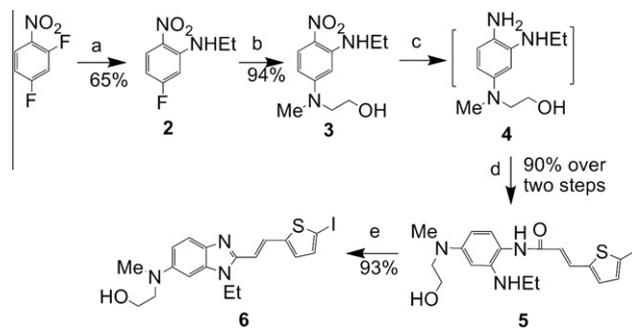
Scheme 1. Reagents and conditions: (a) EtNH<sub>2</sub>, H<sub>2</sub>O, TEA; (b) MeNH(CH<sub>2</sub>)<sub>2</sub>OH, K<sub>2</sub>CO<sub>3</sub>, *N,N*-dimethylacetamide; (c) H<sub>2</sub>, Pd/C, HOAc, THF; (d) 6, TEA, THF; (e) (HOCH<sub>2</sub>)<sub>2</sub>, HOAc, reflux.
