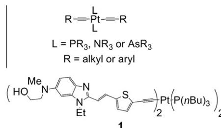
Figure 1. Generic platinum acetylide complex and structure of new molecule 1 synthesized.
