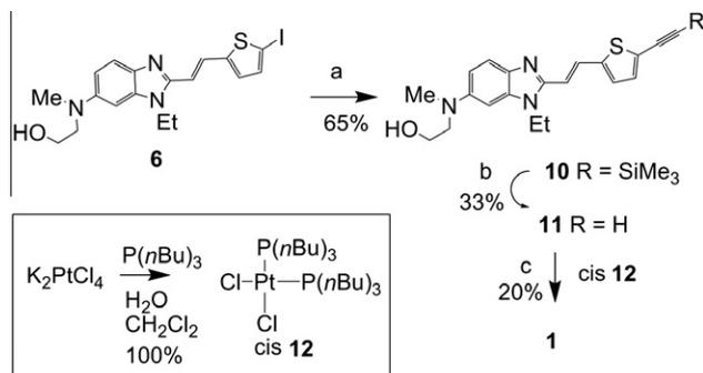
**Scheme 3.** Reagents and conditions: (a) Me<sub>3</sub>SiCCH, Pd(OAc)<sub>2</sub>, PPh<sub>3</sub>, CuI, DIPA, THF, reflux; (b) TBAF, THF; (c) CuI, HN(CH(Me)<sub>2</sub>)<sub>2</sub>, THF.
