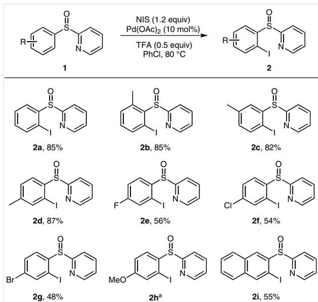
**Scheme 2** Scope of sulfoxide compounds in *ortho*-iodination reactions. All the reactions were carried out in the presence of 0.2 mmol of **1**, 0.22 mmol of NIS and 0.1 mmol of TFA in 1.0 mL PhCl at 80 °C under air conditions. Isolated yields are given. <sup>a</sup> The product could not be isolated in pure form.
