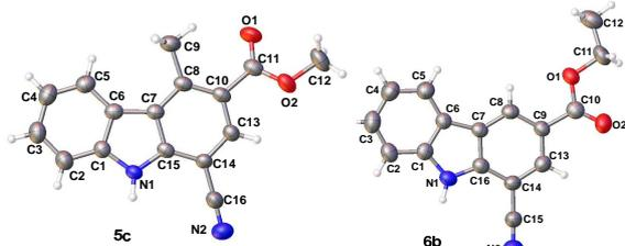
**Figure 2.** X-ray crystallographic structure of **5c** and **6b** with thermal ellipsoid 50% probability level
