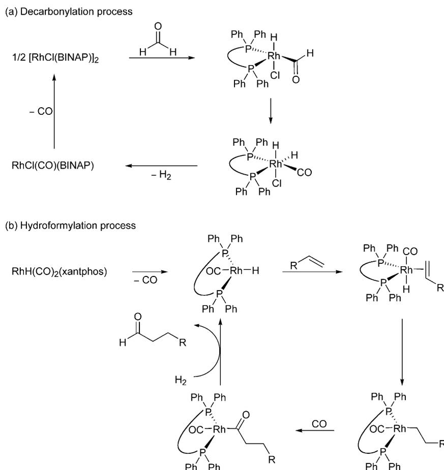
**Scheme 1.** Possible reaction pathway of hydroformylation using formaldehyde catalyzed by two different Rh species.
