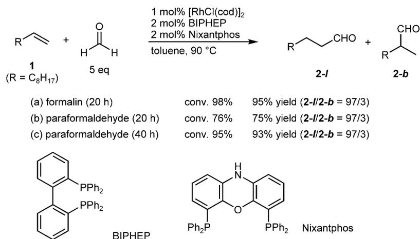
**Scheme 2.** Rh(I)-catalyzed highly linear-selective hydroformylation of 1-decene (**1**) with formaldehyde.
