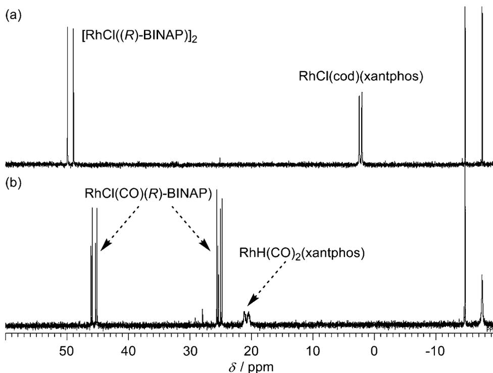
**Figure 1.**  $^{31}\text{P}$  NMR spectra of (a) a mixture of  $[\text{RhCl}(\text{cod})]_2$ , (*R*)-BINAP, and xantphos (1:2:2) in toluene- $d_8$  solution and (b) the reaction of the mixture with formalin.
