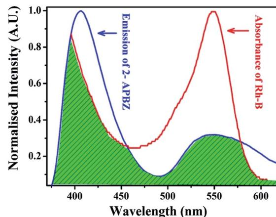
Fig. 4 Overlap spectra of donor emission and acceptor absorbance of L (10  $\mu$ M) in dry acetonitrile.
