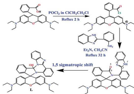
Scheme 1 Synthesis of fluorescence FRET sensor L.
