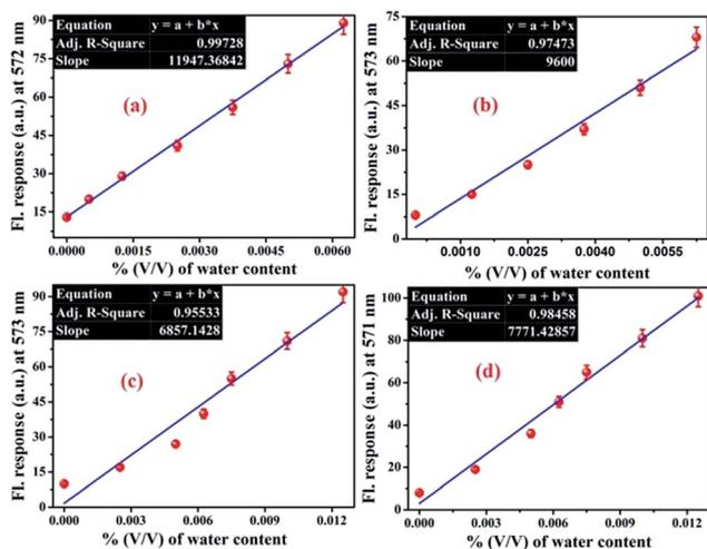
Fig. 2 Calibration curves in the lower concentration range, with error bars for calculating the DL and QL of L as a function of water content in (a) acetonitrile, (b) methanol, (c) DMSO and (d) THF.
