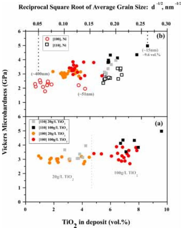
**Fig. 1.** Variation of composites microhardness values with different textures as a function of (a) volume percentage of codeposited nano-TiO<sub>2</sub> particles in nickel matrix and (b) the average grain size ( $d^{-1/2}$ ).
