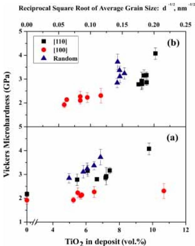
**Fig. 2.** Variation of composites microhardness values with different textures as a function of (a) volume percentage of codeposited nano-TiO<sub>2</sub> particles in nickel matrix and (b) the average grain size ( $d^{-1/2}$ ) [11]. The coatings were produced under an extended region of pulse electrolysis conditions: (■) pH = 4 and  $J_p = 1 \text{ A dm}^{-2}$ , (●) pH = 3.5 and  $J_p = 5 \text{ A dm}^{-2}$ , (▲) pH = 2 and  $J_p = 20 \text{ A dm}^{-2}$ .
