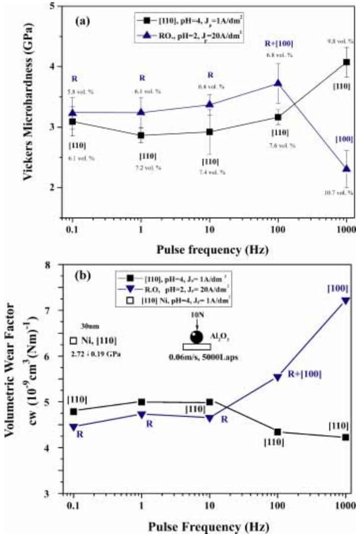
**Fig. 4.** (a) Variation of microhardness values [11] and (b) volumetric wear factor values of composite Ni/nano-TiO<sub>2</sub> coatings prepared under pulse plating conditions as a function of pulse frequency, at a duty cycle of 50%. Composite coatings prepared under the following conditions pH = 4, 2 and  $J_p = 1, 20 A dm^{-2}$ . (Numbers in brackets notify the corresponding nickel preferred orientation of the coating).
