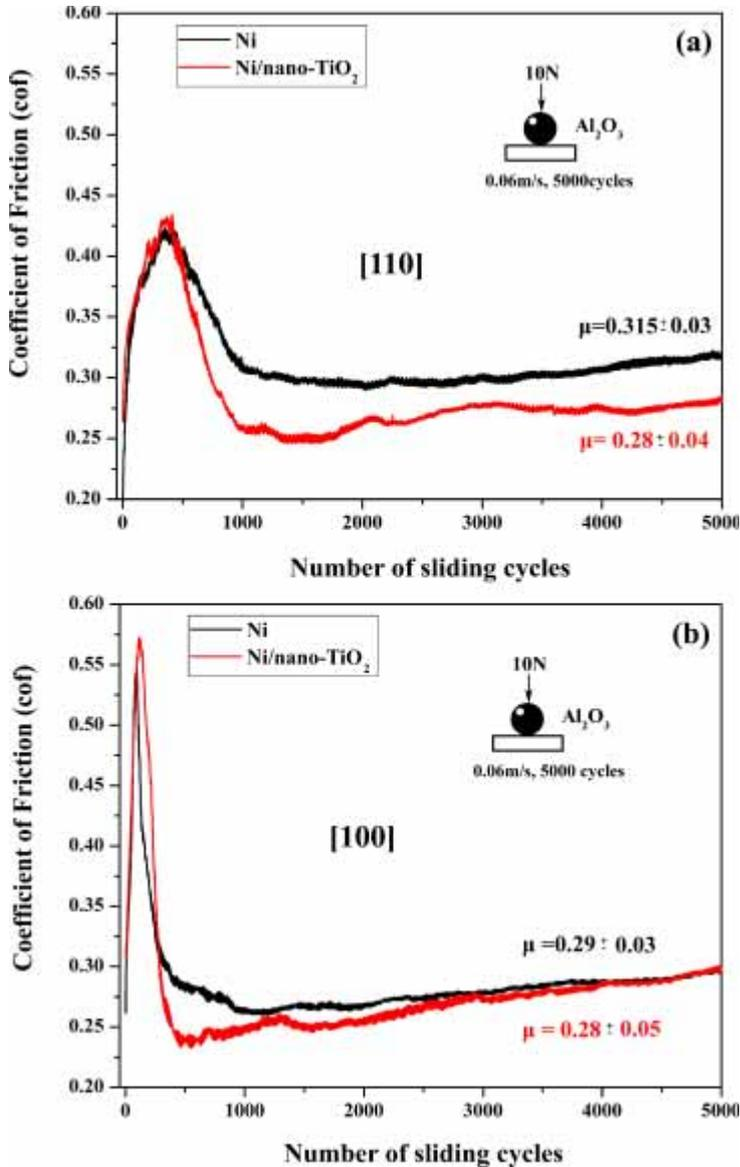
**Fig. 3.** Evolution of friction coefficient for pure Ni and composite Ni/nano-TiO<sub>2</sub> coatings sliding against corundum ball ( $d = 6$  mm), exhibiting (a) the [110] and (b) [100] preferred orientation.
