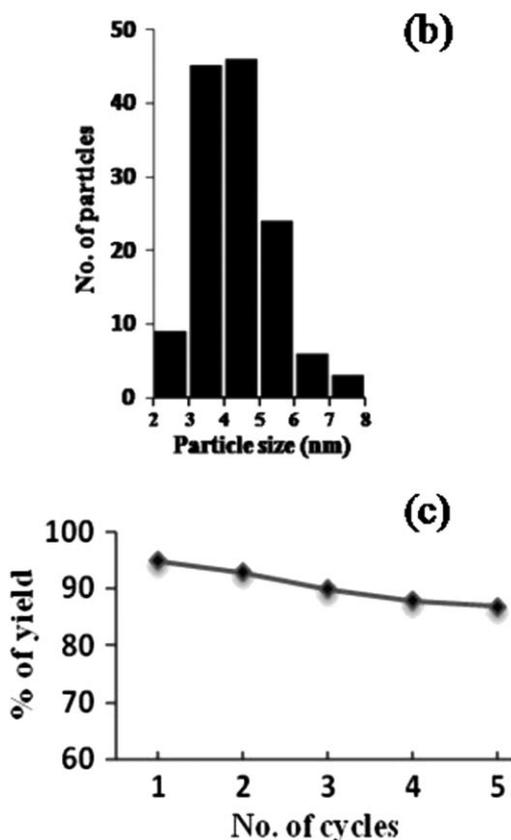
**FIGURE 5** (a) TEM image of Pd@PS after five reaction cycles. (b) histogram showing particle size distribution after five cycles. (c) recyclability results for Pd@PS catalyst
