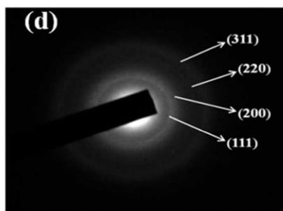
**FIGURE 2** (a) TEM image at 5 nm scale. (b) histogram describing the particle size distribution. (c) high-resolution TEM image showing fast-Fourier transform of marked area. (d) SAED pattern of Pd@PS
