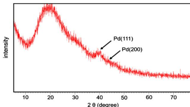
**FIGURE 3** Powder XRD pattern for Pd@PS catalyst
