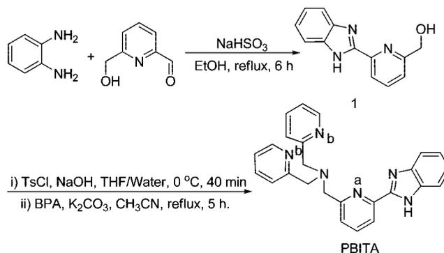
phenylenediamine and 6-(hydroxymethyl)pyridine-2-carbaldehyde in the presence of  $NaHSO_3$  afforded compound **1**, and PBITA was obtained with satisfactory yield by reacting the tosylated derivative of **1** with BPA in  $CH_3CN$  in the presence of  $K_2CO_3$  (Supporting Information).
