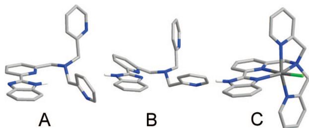
**Figure 4.** Conformations of PBITA optimized by density functional theory calculations: free PBITA (A, B) and  $\text{Zn}^{2+}$ /PBITA complex (C). All of the protons except for the one attached to imidazole N atom are omitted for clarity.
