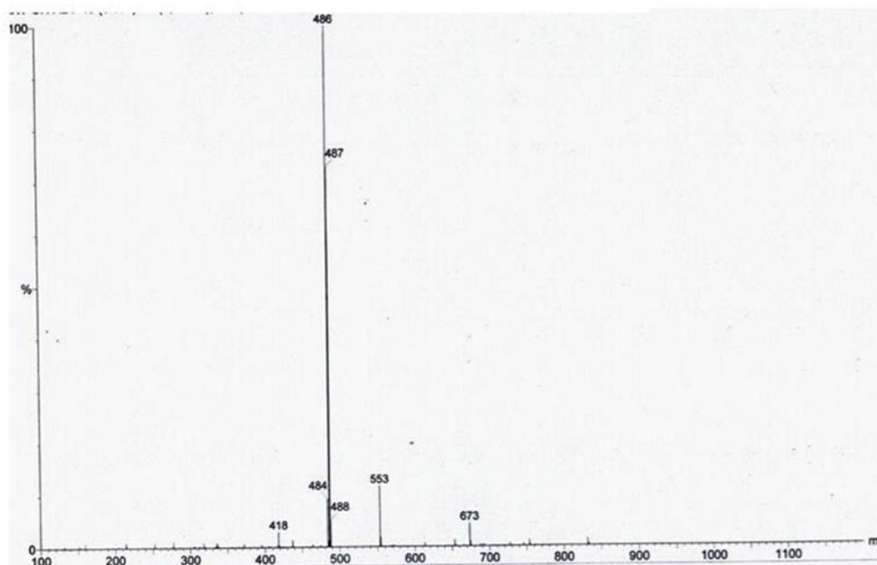
**Fig-4 (b):** ESI-Mass spectrum of  $[\text{CrL}^3(\text{OH}_2)_2]^+$  complex.
