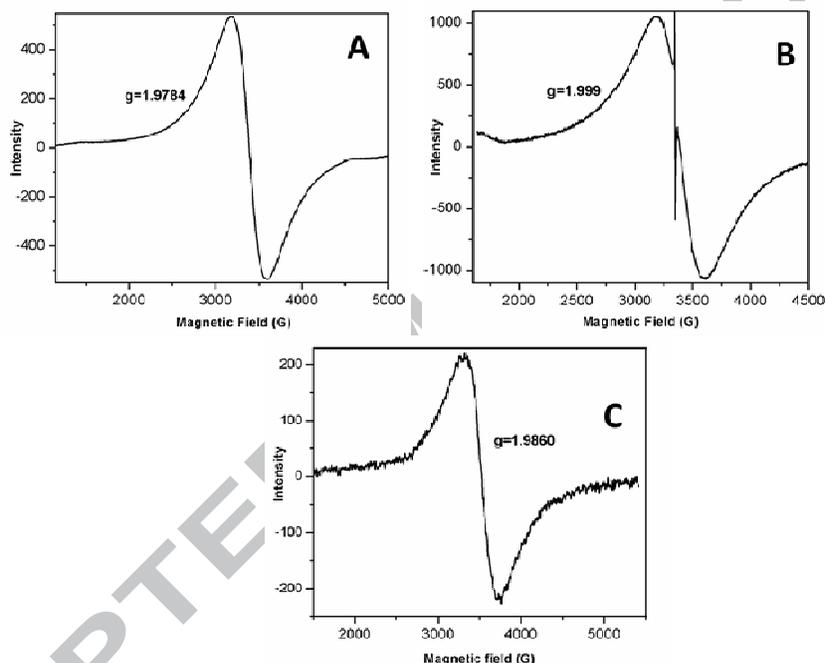
**Fig-5:** EPR spectra of Chromium Schiff base complexes (A)  $[\text{CrL}^1(\text{H}_2\text{O})_2]^+$ ; (B)  $[\text{CrL}^3(\text{H}_2\text{O})_2]^+$ ; (C)  $[\text{CrL}^4(\text{H}_2\text{O})_2]^+$ .
