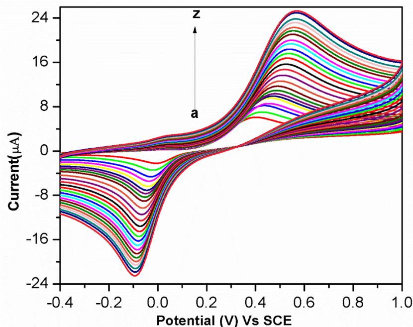
**Fig-8:** Cyclic voltammograms of  $[\text{CrL}^2(\text{H}_2\text{O})_2]^+/\text{GCE}$  in  $1 \times 10^{-4}$  M CT (pH 7.0) at the scan rate of (a) 10, (b) 20, (c) 30, (d) 40, (e) 50, (f) 60, (g) 70, (h) 80, (i) 90, (j) 100, (k) 125, (l) 150, (m) 175, (n) 200, (o) 225, (p) 250, (q) 275, (r) 300, (s) 325, (t) 350, (u) 375, (v) 400, (w) 425, (x) 450, (y) 375 and (z)  $500 \text{ mVs}^{-1}$ .
