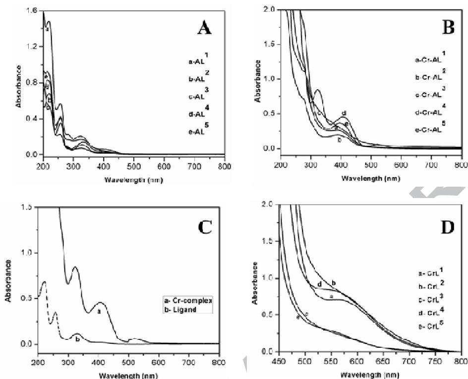
**Fig-2:** (A) UV-Visible spectra of Schiff base, (B) UV-Visible spectra of chromium Schiff base complexes, (C) Comparison UV-Visible spectra of Schiff base and its chromium complex and (D) UV- Visible spectrum for d-d transition.
