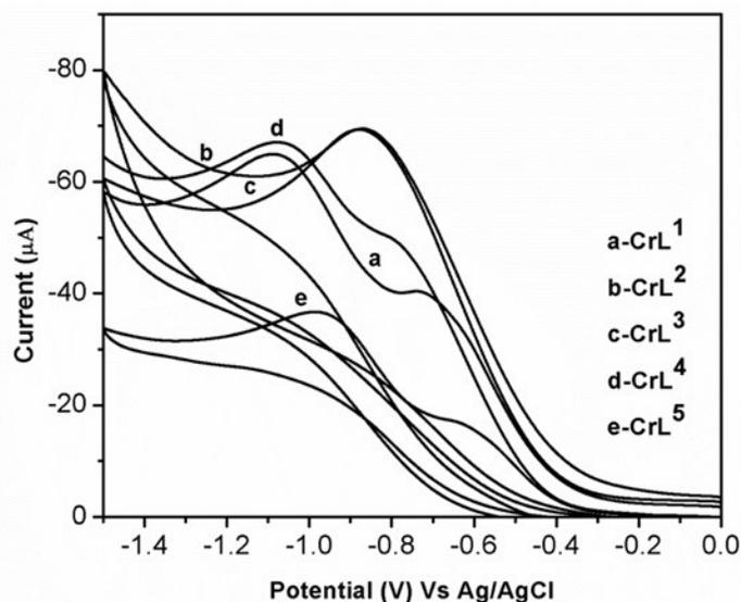
**Fig-6:** Cyclic voltammograms of chromium complexes in acetonitrile at the scan rate of  $50 \text{ mVs}^{-1}$ .
