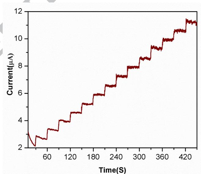
**Fig - 10:** Chronoamperometric responses of  $[\text{CrL}^2(\text{H}_2\text{O})_2]^+/\text{GCE}$  for the successive additions of 5  $\mu\text{L}$  of  $1 \times 10^{-4}$  M CT to 30 mL of 0.1 M PBS. Applied potential is 0.38 V.
