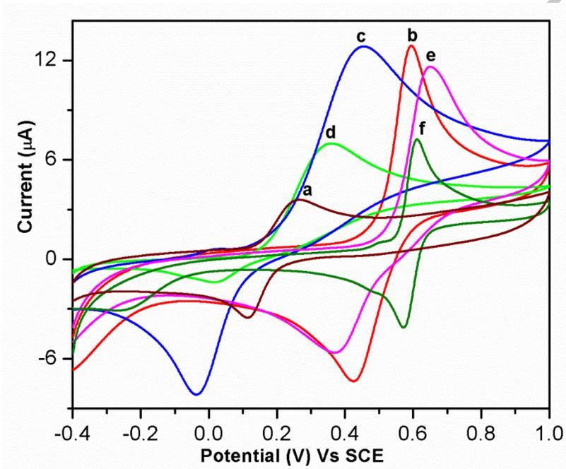
**Fig-7:** Cyclic voltammograms of (a) bare GCE, (b)  $[\text{CrL}^1(\text{H}_2\text{O})_2]^+/\text{GCE}$ , (c)  $[\text{CrL}^2(\text{H}_2\text{O})_2]^+/\text{GCE}$ , (d)  $[\text{CrL}^3(\text{H}_2\text{O})_2]^+/\text{GCE}$ , (e)  $[\text{CrL}^4(\text{H}_2\text{O})_2]^+/\text{GCE}$  and (f)  $[\text{CrL}^5(\text{H}_2\text{O})_2]^+/\text{GCE}$  in presence of  $1 \times 10^{-4}$  M CT at scan rate of  $50 \text{ mV s}^{-1}$
