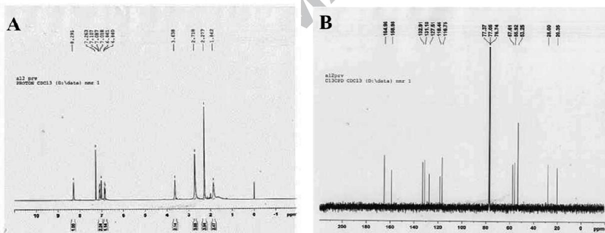
**Fig. 3:** (A) and (B) are  $^1\text{H}$  and  $^{13}\text{C}$  NMR Spectra of  $\text{H}_2\text{L}^2$
