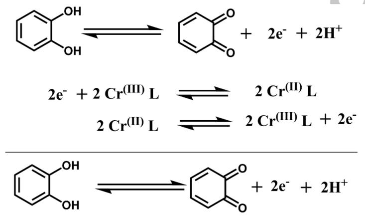
Scheme – 3: Electrocatalytic redox reaction of catechol (CT)
