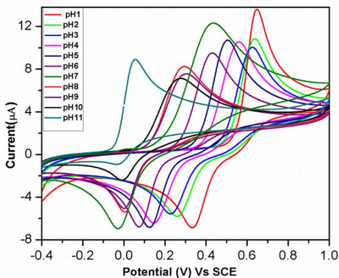
Fig – 9: CVs of  $1 \times 10^{-4} \text{ M}$  CT in different pH value from 1 to 11 on  $[\text{CrL}^2(\text{H}_2\text{O})_2]^+ / \text{GCE}$ .
