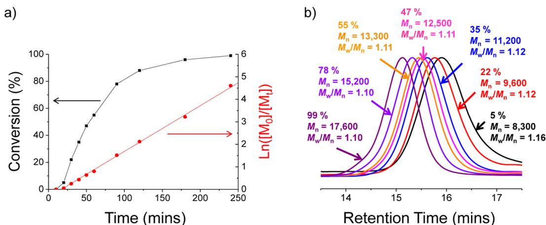
**Figure 4.** Kinetic data obtained for the synthesis of PGMA macro-CTA. A DP of 45 was targeted and a CTA/initiator molar ratio of 5.0 was utilized at 70 °C in aqueous solution: (a) conversion vs time curve (black squares) and the corresponding semi-logarithmic plot (red circles); (b) DMF GPC curves obtained with corresponding conversions, as judged by  $^1\text{H}$  NMR spectroscopy.
