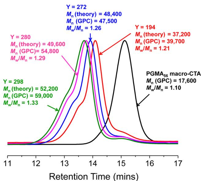
**Figure 5.** DMF GPC curves obtained for a series of PGMA<sub>56</sub>–PPHMA<sub>y</sub> diblock copolymers (where y varies from 194 to 298) and the corresponding PGMA<sub>56</sub> macro-CTA.
