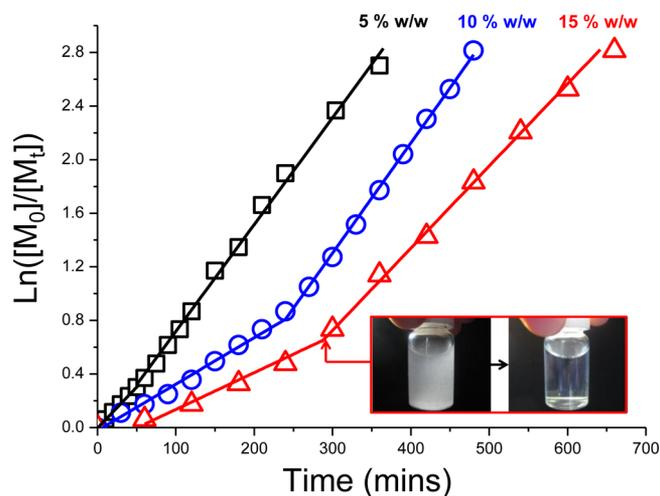
**Figure 2.** Rate of hydrolysis of glycidyl methacrylate (GlyMA) to form glycerol monomethacrylate (GMA) in water at 80 °C in the presence of air at three different GlyMA concentrations, as judged by <sup>1</sup>H NMR spectroscopy. A significant rate enhancement is observed in each case, the onset of which corresponds to the point in the reaction at which sufficient GMA is generated to transform the initial two-phase emulsion into a homogeneous aqueous solution (see inset).
