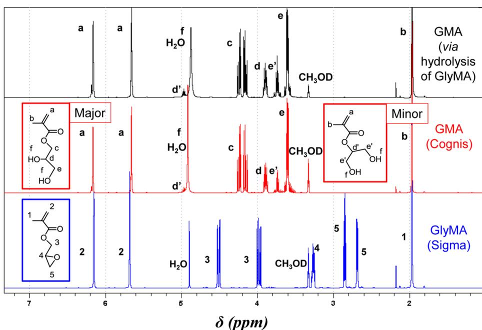
**Figure 1.** <sup>1</sup>H NMR spectra (CD<sub>3</sub>OD) of glycerol monomethacrylate (GMA) monomer prepared via hydrolysis of glycidyl methacrylate (GlyMA) at 10% w/w (upper spectrum), commercial GMA monomer donated by Cognis (middle spectrum), and commercial glycidyl methacrylate monomer (lower spectrum).
