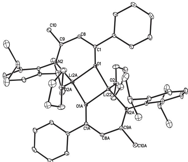
**Fig. 1.** ORTEP diagram of complex  $\text{Li}_2(\text{L}^{2,6\text{-ipr}})_2 \cdot 2(\text{THF})$  **8** showing an atom numbering scheme. Thermal ellipsoids are drawn at the 30% probability level and hydrogen atoms are omitted for clarity (#1  $-x + 1, -y + 1, -z + 2$ ).
