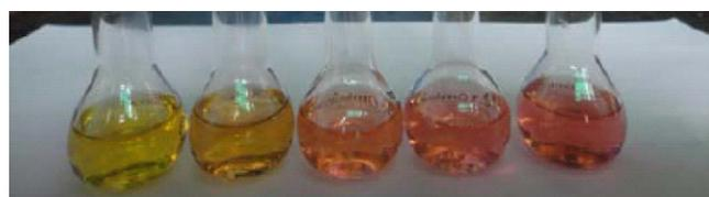
Fig. 2. Photographs of **L** color changes (10.0  $\mu\text{M}$ ) with gradual addition of  $\text{Ni}^{2+}$  from left to right: 0, 4, 10, 20 and 50  $\mu\text{M}$ , respectively in  $\text{CH}_3\text{CN}$  solution.
