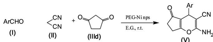
**Scheme 2.** PEG-stabilized Ni nanoparticles catalyzed the synthesis of tetrahydro-cyclopenta[b]pyran derivatives.
