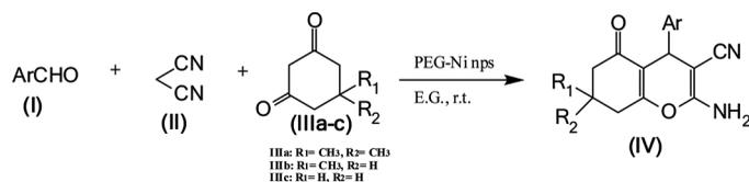
**Scheme 1.** PEG-stabilized Ni nanoparticles catalyzed the synthesis of tetrahydro-4H-benzo[b]pyran derivatives.
