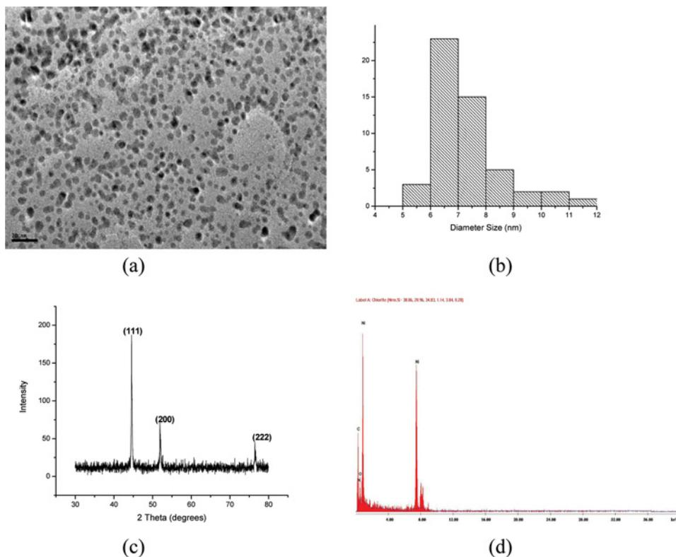
**Figure 1.** (a) TEM image of PEG-Ni nanoparticles; (b) size histogram of PEG-Ni nanoparticles; (c) x-ray diffraction pattern of PEG-Ni nanoparticles; and (d) EDAX data of PEG-Ni nanoparticles. (Figure is provided in color online.)
