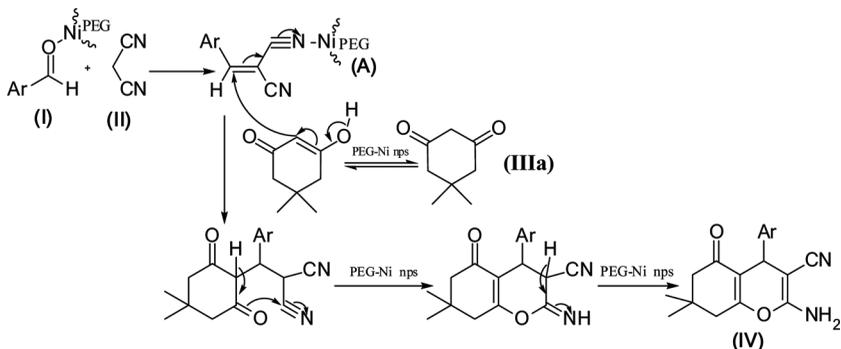
**Scheme 5.** Plausible mechanistic pathway for the PEG-Ni nanoparticle-catalyzed synthesis of 4*H*-pyrans.
