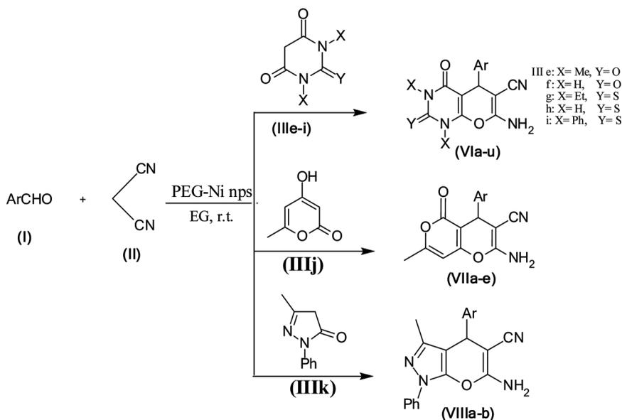
**Scheme 3.** PEG-stabilized Ni nanoparticles catalyzed the synthesis of 2-amino-4-aryl-4*H*-pyran-3-carbonitrile derivatives.
