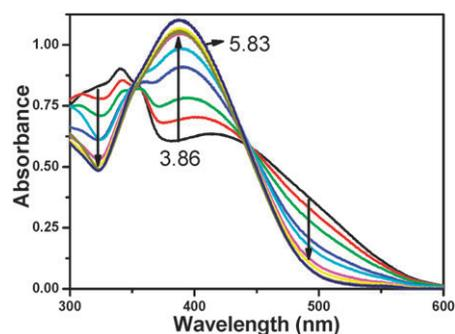
**Fig. 5** Absorption spectra of **BTP** ( $5 \times 10^{-6} \text{ M}$ ) in aqueous solutions (MeOH-water, 1:99, v/v) at different pH values. The arrows display the variation of absorbance from pH 3.86 to 5.83.
