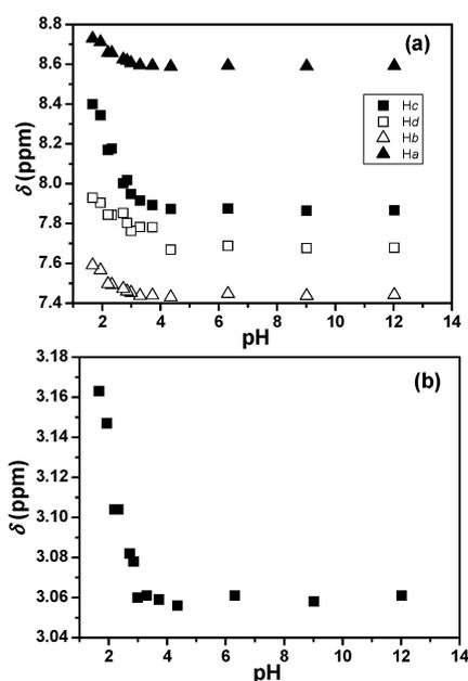
**Fig. 4** pH Titration profiles of **BTP** according to the chemical shifts of the pyridine protons (a) and *N,N*-dimethylamine protons (b) at different pH values (pH values were converted from pD by  $\text{pH} = \text{pD} - 0.4$ ).<sup>23</sup>
