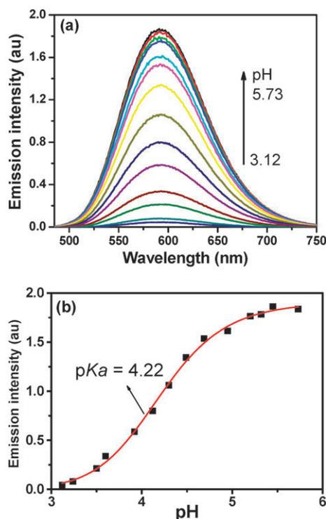
**Fig. 1** (a) Emission spectra of **BTP** ( $5 \times 10^{-6}$  M) in aqueous solutions (MeOH–water = 1:99, v/v) at different pH, (b) emission intensity at 597 nm versus pH in acidic conditions according to the fluorescent pH titration.  $\lambda_{\text{ex}} = 397$  nm.
