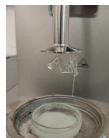
Figure 5. Adhesive film of 3 after the tack test.
