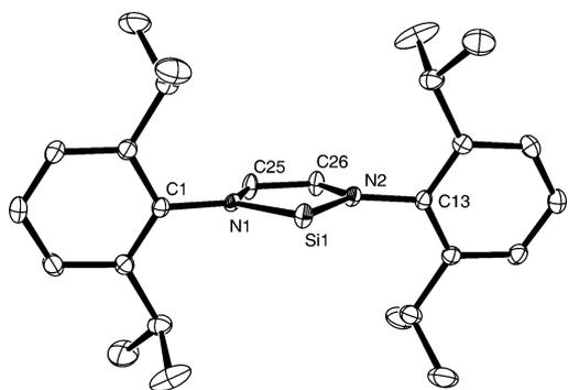
**Fig. 2** Ortep drawing of **5** with 30% probability. Hydrogen atoms have been omitted for clarity. Selected bond lengths (Å) and angles (deg): Si1–N1 1.761(4), Si1–N2 1.774(4), C25–N1 1.420(4), C26–N2 1.379(4), C25–C26 1.391(7) N1–Si1–N2 87.50(17), C25–N1–Si1 113.4(3), C26–N2–Si1 114.9(3), C25–C26–N2 111.9(3), C26–C25–N1 112.3(3), C1–N1–C25 118.9(3), C1–N1–Si1 127.8(3), C13–N2–Si1 127.4(2).
