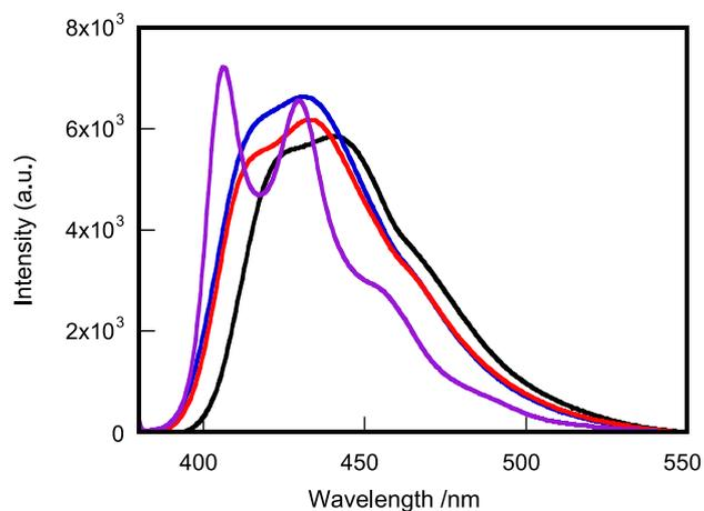
**Figure 3.** Fluorescence spectra of **5a** in DMSO (black), cyclohexane (purple), acetone (red), and methanol (blue);  $c=10 \mu\text{M}$ .
