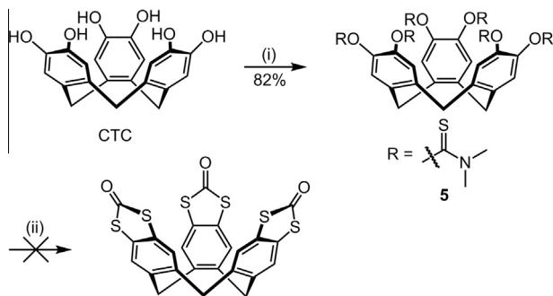
**Scheme 2.** Attempted Newman–Kwart rearrangement from pre-formed cyclotriicatechylene. Reagents and conditions: (i)  $\text{Me}_2\text{NC}(\text{S})\text{Cl}$ ,  $\text{Cs}_2\text{CO}_3$ , DMF; (ii)  $\text{Ph}_2\text{O}$ ,  $180^\circ\text{C}$ .
