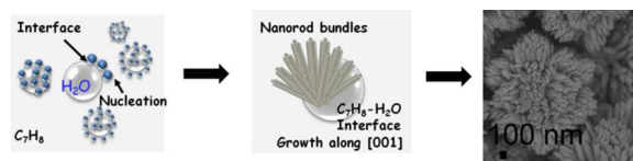
Scheme 1. Proposed mechanism of the self-assembly to produce the rutile \text{TiO}_2 nano-flower hierarchical structures.
