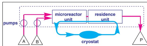
**Figure 1** Schematic design of a CPC microstructured flow-through reactor (Cytos): two stock solutions (A and B) are pumped through a microstructured mixing and reaction unit cooled by a cryostat
