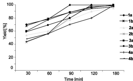
Figure 5. Time dependence of the catalytic transfer hydrogenation of cyclohexanone; catalyst (**1a–4b**; 0.02 mmol), KOH (0.2 mmol), cyclohexanone (4 mmol), and 2-propanol (20 mL),  $T = 353$  K.
