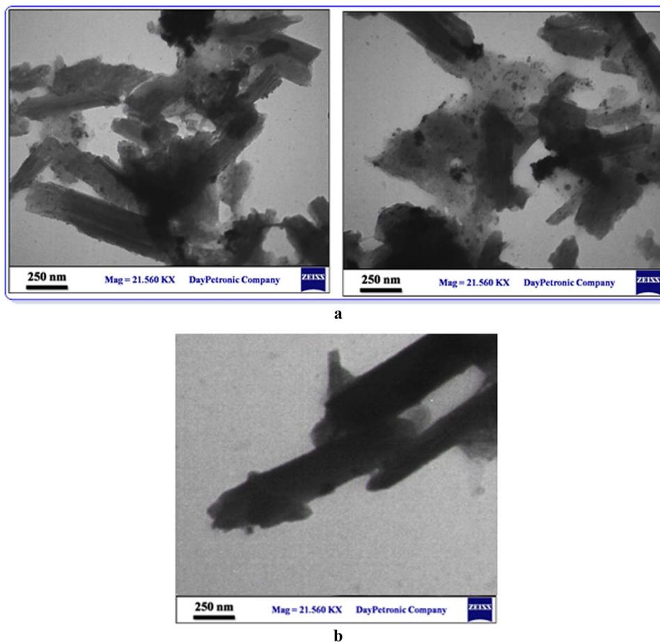
Fig. 2. a: TEM images of the catalyst and b: the TEM image of the pristine Hal.
