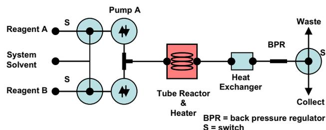
Figure 1. Schematic representation of the flow apparatus.
