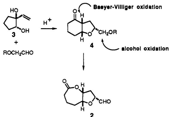
of marine natural products from a common bicyclic lactone aldehyde precursor **2**. This intermediate embodies the three stereogenic centers of the central tetrahydrofuran ring and also provides loci for the elaboration of the remaining six carbons of these halogenated lipid targets.
