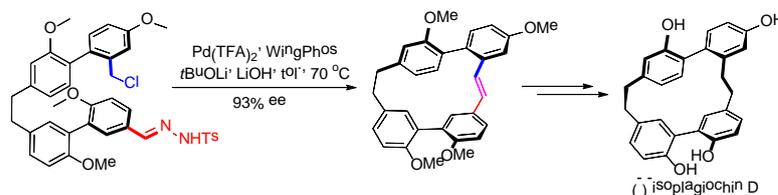
A catalytically asymmetric macrocyclization via palladium-catalyzed intramolecular coupling between benzyl chloride and arylhydrazone was reported. This method enabled the asymmetric total synthesis of bisbibenzylis isoplagiochin D.
