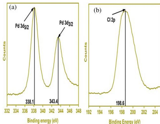
**FIGURE 3** Binding energy (eV) plots for (a) palladium and (b) chlorine in Pd-PEPPSI-3 XPS spectroscopy
