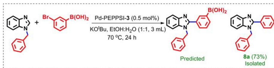
**SCHEME 5** Investigation on functional groups tolerance of Pd-PEPPSI-3 for halide partner. Reaction conditions: benzimidazole (1.0 mmol), 3-bromo phenylboronic acid (1.0 mmol), KO<sup>t</sup>Bu (3.0 mmol), Pd-PEPPSI-3 (0.5 mol%), EtOH-water (1:1, 3 ml), 70 °C, 24 h
