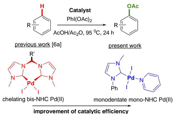
**Fig. 1.** Development of Pd(II)-NHC catalyst for non-directed arene C-H acetoxylation
