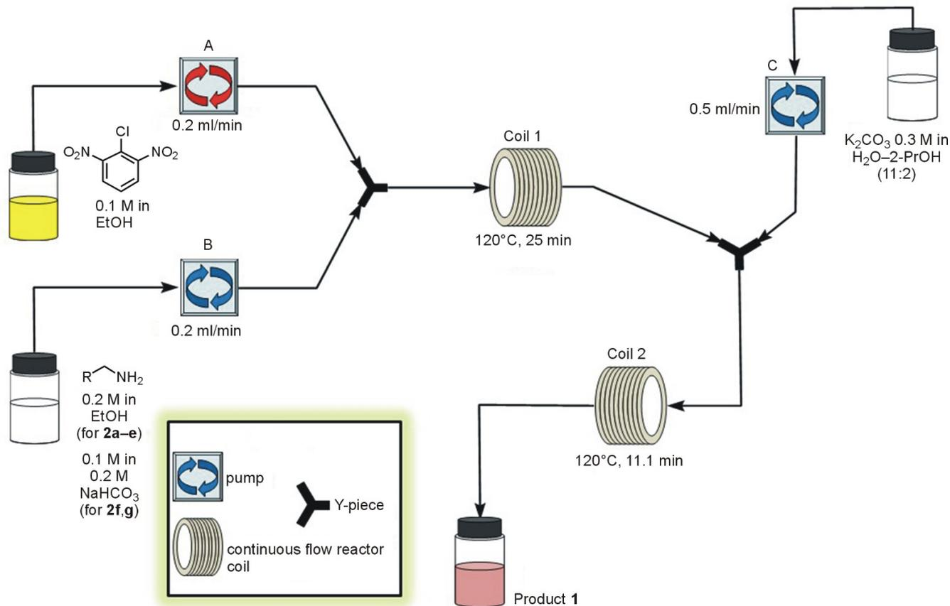
**Figure 2.** The flow configuration used for the preparation of nitrobenzimidazole *N*-oxides **1** in flow.
