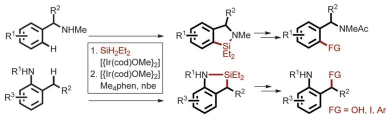
**A'SiN'ch:** In the title reaction of benzylamines or anilines, (hydrido)silyl amines are generated in situ which undergo selective silylation at the C–H bond  $\gamma$  to the amino group. The silylation products
