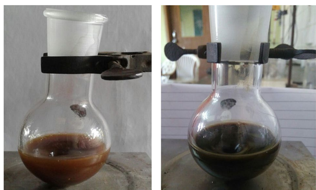
A At starting (Extract + Pd(OAc) 2 ) B After formation (Extract + Pd NPs)
