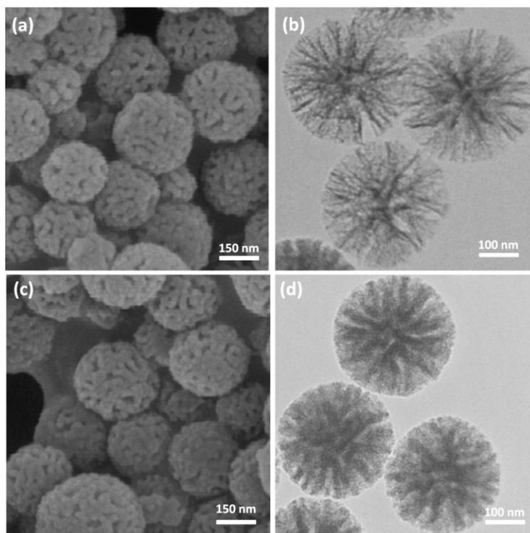
**Figure 1** FESEM images of KCC-1 NPs (a); TEM images of KCC-1 NPs (b); FESEM images of KCC-1/Pd-NHC-Py NPs (c); TEM images of KCC-1/Pd-NHC-Py NPs (d).
