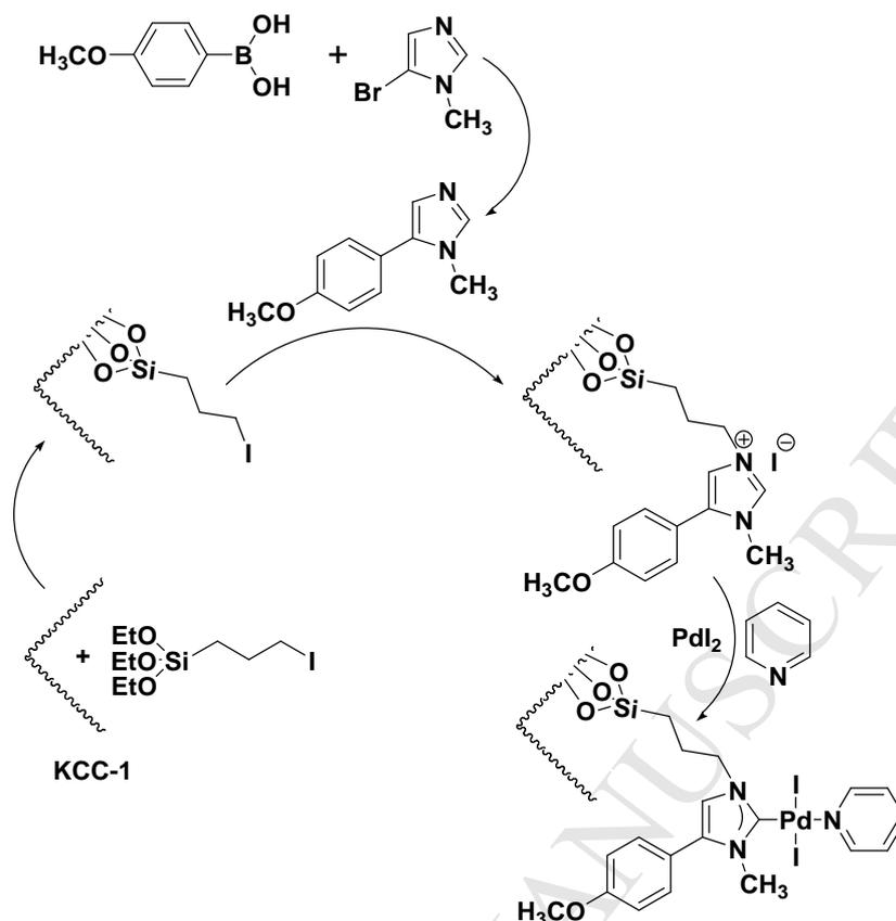
**Scheme 2** Schematic illustration of the synthesis for KCC-1/Pd-NHC-Py NPs.
