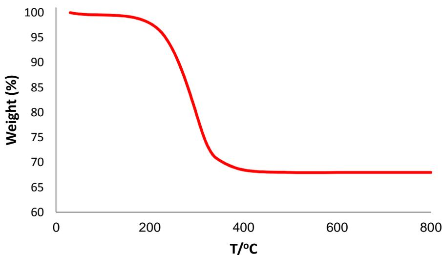
**Figure 3** TGA diagram of KCC-1/Pd-NHC-Py NPs.
