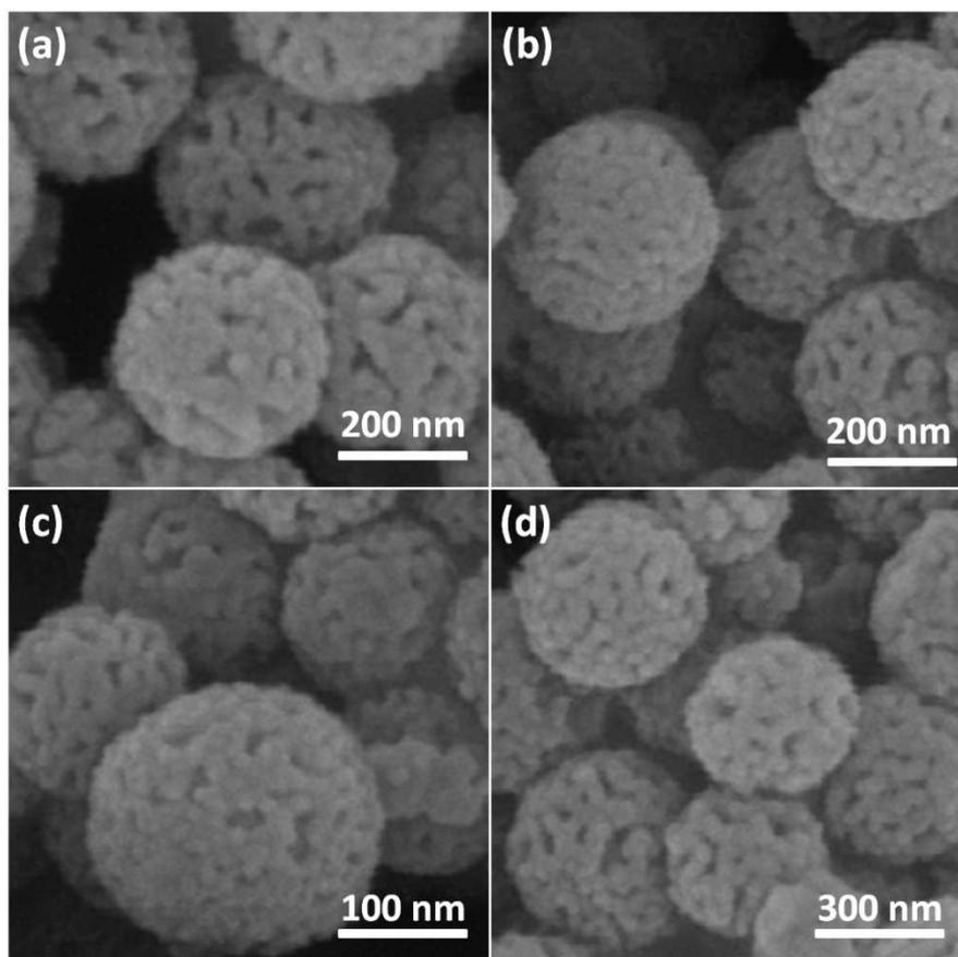
**Figure 2** FESEM images of KCC-1/Pd-NHC-Py NPs after mechanical compression at pressures of 200 Mpa (a); after microwave irradiation at power to 650 W (b); after heating in boiling DMSO for 60 h (c); after calcination at 1000 °C/6 h (d).
