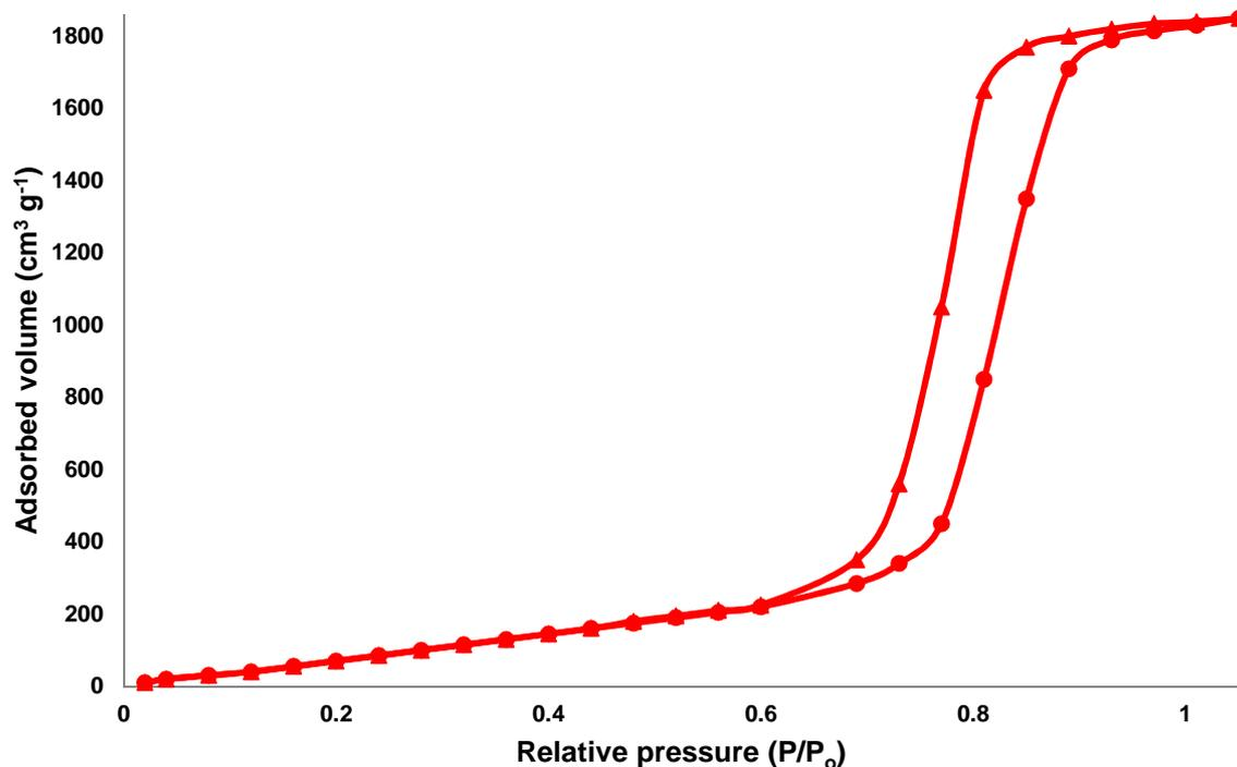
**Figure 4** Adsorption–desorption isotherms of KCC-1/Pd-NHC-Py NPs.
