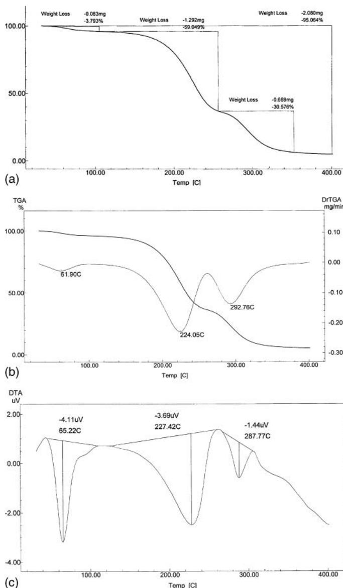
FIG. 3. (a) TGA of phosphorylated product (7); (b) DTGA of phosphorylated product (7); (c) DTA of phosphorylated product (7).
