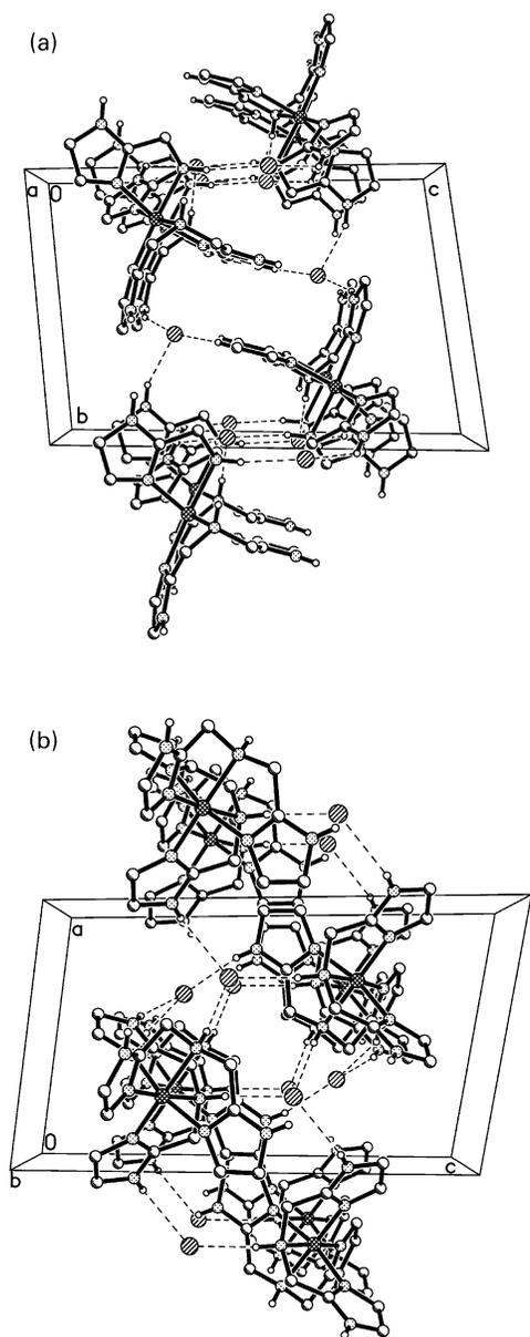
Fig. 2. The packing diagram of the title complex viewed along (a) *a*-axis and (b) *b*-axis. Hydrogen bonds are shown as dotted lines and H atoms not involved in hydrogen bonding and phenyl rings have been omitted for clarity.
