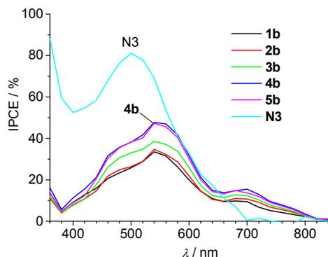
Fig. 7 The IPCE characteristics of DSSCs with **1b** – **5b** and **N3**.
