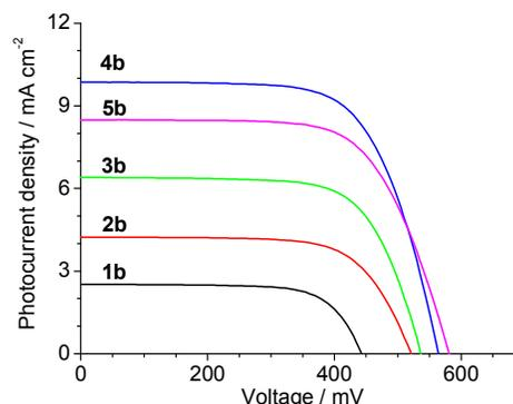
**Fig. 6** Photocurrent density-voltage characteristic of devices using cyclometalated ruthenium sensitizers.
