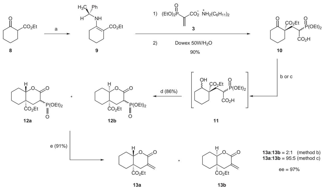
**Scheme 2** Reagents and conditions: a. (*S*)-1-Phenylethylamine, *p*TSA (cat.), toluene, reflux, 8 h; b. EtOH, KOH (1 equiv),  $\text{KBH}_4$  (1 equiv), r.t., 24 h; c. MeOH,  $\text{CeCl}_3 \cdot 7\text{H}_2\text{O}$  (1 equiv),  $\text{KBH}_4$  (1 equiv),  $-70^\circ\text{C}$ , 1 h, r.t., 24 h; d. *p*TSA (cat.), benzene, reflux, 4 h; e. *t*-BuOK (1.1 equiv),  $(\text{HCHO})_n$  (5 equiv),  $\text{Et}_2\text{O}$ , r.t., 1 h.
