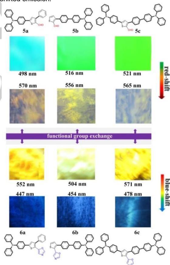
**Figure 2.** The fluorescent images of **5** and **6** before and after grinding.
