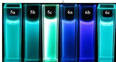
**Figure 1.** Fluorescence images of **5a–5c** and **6a–6c** in toluene ( $5.0 \times 10^{-5}$  M) under UV light (365 nm).
