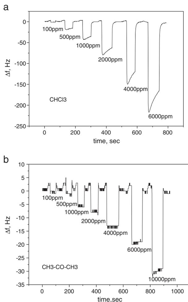
Fig. 3. Kinetic responses of the QCM sensors covered with calixarene **5a** (30 monolayers) to sorption of chloroform (a) and acetone (b) at different concentrations in air.
