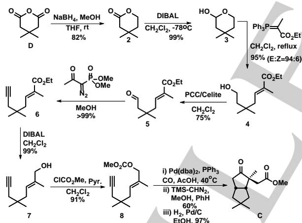
Scheme 2. Stereoselective synthesis of diquinane intermediate **C**.
