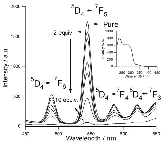
**Fig. 2.** Emission spectra of  $\text{Tb}(\mathbf{a})_3$  ( $10^{-5}$  M in acetonitrile,  $\lambda_{\text{ex}} = 284$  nm) upon addition of 0–10 equivalents of  $[\text{Bu}_4\text{N}]\text{F}$ . Insert: excitation spectra of  $\text{Tb}(\mathbf{a})_3$  ( $10^{-5}$  M in acetonitrile,  $\lambda_{\text{em}} = 544$  nm).
