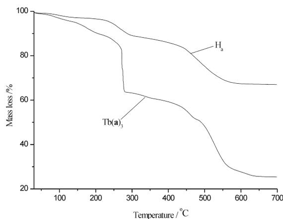
**Fig. 5.** Thermogravimetric analysis of  $\text{Tb}(\mathbf{a})_3$  and  $H_a$ .
