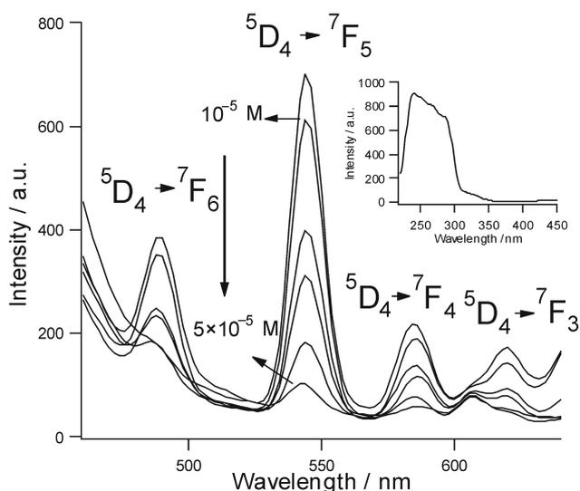
**Fig. 4.** Emission spectra of  $H_a$  ( $0.5 \text{ mg mL}^{-1}$  in water,  $\lambda_{\text{ex}} = 290 \text{ nm}$ ) upon addition of  $0\text{--}5 \times 10^{-5} \text{ M}$   $[\text{Bu}_4\text{N}]\text{HSO}_4$ . Inset: Excitation spectra of  $H_a$  ( $0.5 \text{ mg mL}^{-1}$  in water,  $\lambda_{\text{em}} = 544 \text{ nm}$ ).
