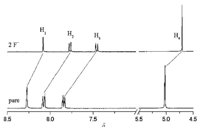
**Fig. 3.**  $^1\text{H}$  NMR spectra measured by titration of a DMSO- $d_6$  solution of pure **a** (1 mM) with two equivalents of  $[\text{Bu}_4\text{N}]\text{F}$ .
