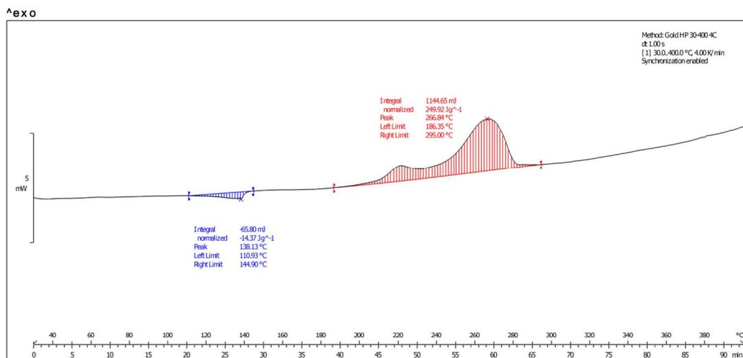
**Figure 1: Differential scan calorimetry (DSC) chart of Krapcho decarboxylation (4.5 mg reaction mixture)**
