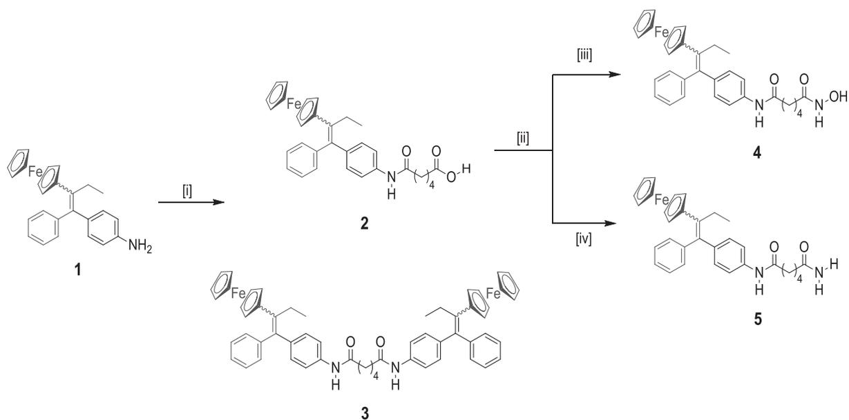
**Scheme 1.** Synthesis of adipic derivatives. Reagents and conditions: [i]  $(\text{ClCOCH}_2\text{CH}_2)_2$ , DCM, rt, 20 min (51%). [ii]  $\text{ClCO}_2\text{Et}$ , TEA, THF,  $0^\circ\text{C}$ , 15 min [iii]  $\text{NH}_2\text{OH}\cdot\text{HCl}$ , KOH, MeOH,  $0^\circ\text{C}$ , 20 min then 2.5 h (36%). [iv]  $\text{NaNH}_2$ , rt, 30 min (93%).
