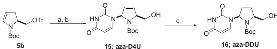
**Scheme 3.** Reagents and conditions: (a) i.  $(\text{TMS})_2\text{-uracil}$ ,  $\text{PhSeBr}$ ,  $\text{CH}_3\text{CN}$ ,  $-23^\circ\text{C}$ ; ii.  $\text{ZnBr}_2$ ,  $\text{MeOH}$ ,  $\text{CH}_2\text{Cl}_2$ ; (b)  $\text{H}_2\text{O}_2$ , dioxane,  $\text{NaHCO}_3$ ; (c)  $\text{H}_2$ ,  $\text{Pd/C}$ ,  $\text{EtOAc}$ .
