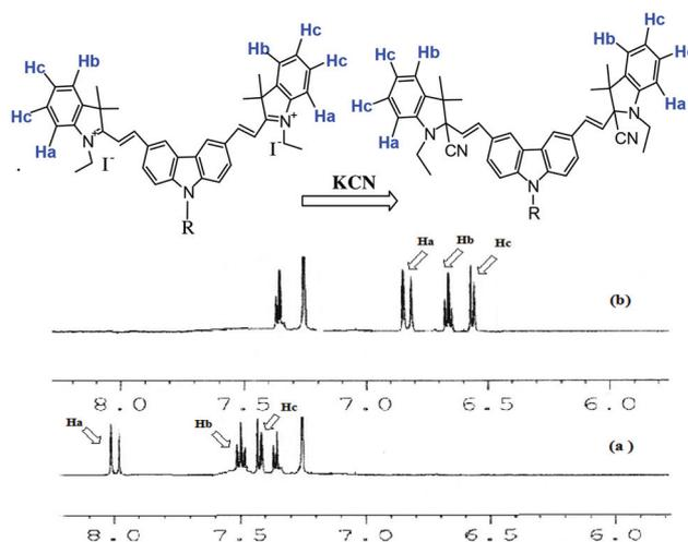
**Fig. 7**  $^1\text{H-NMR}$  spectra of (a) CHD and (b) CHD +  $\text{CN}^-$  in  $\text{CDCl}_3$ .
