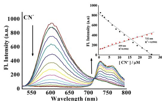
**Fig. 2** Titration spectra of CHD ( $c = 2.0 \times 10^{-5}\text{ M}$ ) in the presence of 2 equiv. of  $CN^-$  ( $c = 2.0 \times 10^{-4}\text{ M}$ ) at pH 7.1 in  $CH_3CN$ - $H_2O$  (1 : 1, v/v) and plot of  $[CN^-]$  vs. Fl. Intensity at two different wavelengths.
