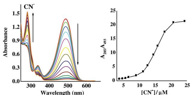
**Fig. 1** UV-vis absorption titration spectra of CHD ( $c = 2.0 \times 10^{-5}\text{ M}$ ) in the presence of 2 equiv. of  $CN^-$  ( $c = 2.0 \times 10^{-4}\text{ M}$ ) at pH 7.1 in  $CH_3CN$ - $H_2O$  (1 : 1, v/v) (left) and absorbance ratio changes ( $A_{285}/A_{493}$ ) of CHD upon gradual addition of  $CN^-$  (2 equiv.) (right).
