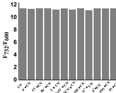
**Fig. 5** Fluorescence responses of CHD ( $c = 2.0 \times 10^{-5} \text{ M}$ ) to  $\text{CN}^-$  (2 equiv.) containing 10 equiv. of various anions.  $\lambda_{\text{ex}} = 250 \text{ nm}$  (right).
