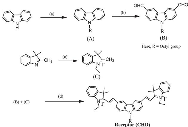
**Scheme 1** Synthetic route to CHD. Reagents and conditions: (a) octylbromide,  $K_2CO_3$ , KI,  $CH_3CN$ , heated at  $80\text{ }^\circ\text{C}$ , 4 h; (b)  $POCl_3$ , DMF,  $100\text{ }^\circ\text{C}$ , 20 h; (c) ethyl iodide, toluene, reflux, 8 h; (d) ethanol, piperidine (cat), reflux, 12 h.
