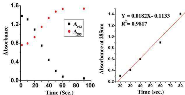
**Fig. 3** Time-dependent absorption intensity of CHD at 285 nm (in red) and 493 nm (in black) in the presence of  $\text{CN}^-$  (2 equiv.) (left) and the time vs. absorbance at a fixed wavelength (285 nm) plot using the first order rate equation (right).
