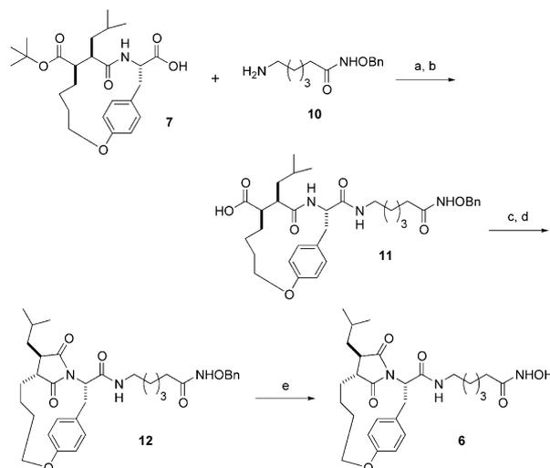
**Scheme 2.** Reagents and conditions: (a) EDC, HOBT, NMM, DMF; (b) TFA, CH<sub>2</sub>Cl<sub>2</sub>, 93% two steps; (c) *i*PrO<sub>2</sub>CCl, Et<sub>3</sub>N, DMF, 0 °C; MeOH, 93%; (d) KO*t*Bu, THF, 76%; (e) H<sub>2</sub>, Pd/C, THF, 94%.
