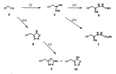
**Reagents:** (i) NaOMe, MeOH; (ii)  $CH_3CO_2H$ , NH<sub>2</sub>NHCHO; (iii)  $CH_3CO_2H$ , NH<sub>2</sub>NHCO<sub>2</sub>Me; (iv) AlCl<sub>3</sub>, NaN<sub>3</sub>, THF, reflux; (v)  $CH_2N_2$ ,  $Et_2O$ ,  $0^{\circ}C$ .
